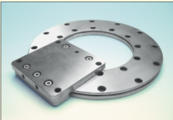
Frictionless ringslides type RPM (stainless steel). They allow the user a precision curved movement, almost free of friction and pre-loaded. Ball diameter 3 mm. Rotating range max 360°.
