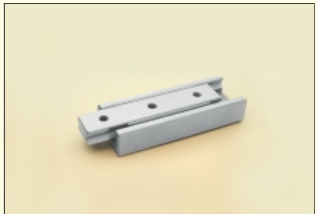
Miniature precision stainless steel ball slide type PMM . Strokelength 5–70 mm. In 3 sizes available. Weight 2–70 grams. For rapid and precise linear motions.
