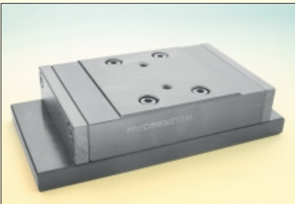
Dust-protected roller table type RTNG (steel /cast-iron). Strokelength 10–250 mm. Max. loadcapacity 35.100 N.
