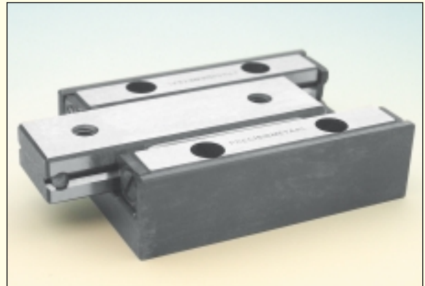
Low profile crossed roller table type RTS (steel). Strokelength 12–130 mm. Max. loadcapacity 3.672 N
